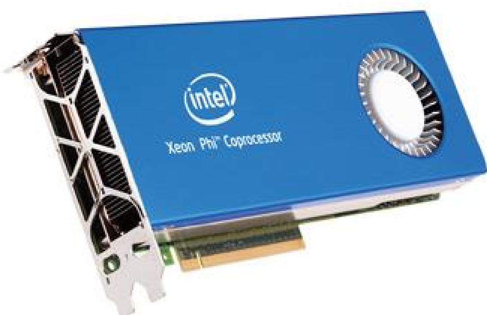
Figure 1. Intel Xeon Phi coprocessor (aka MIC). Specs: • ~60 cores • 4 hardware threads per core • 8-16 GB GDDR5 memory • 512-bit vector registers • over 1 teraFLOPs double-precision peak performance
