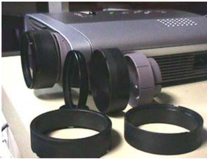
**Figure 11. Polarization filter and mount.**
