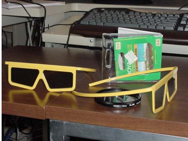
**Figure 17. Glasses with circular polarization.**
