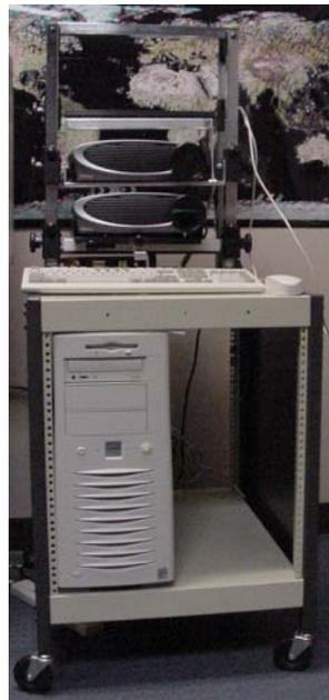
**Figure 3. The portable Geowall computer.**
